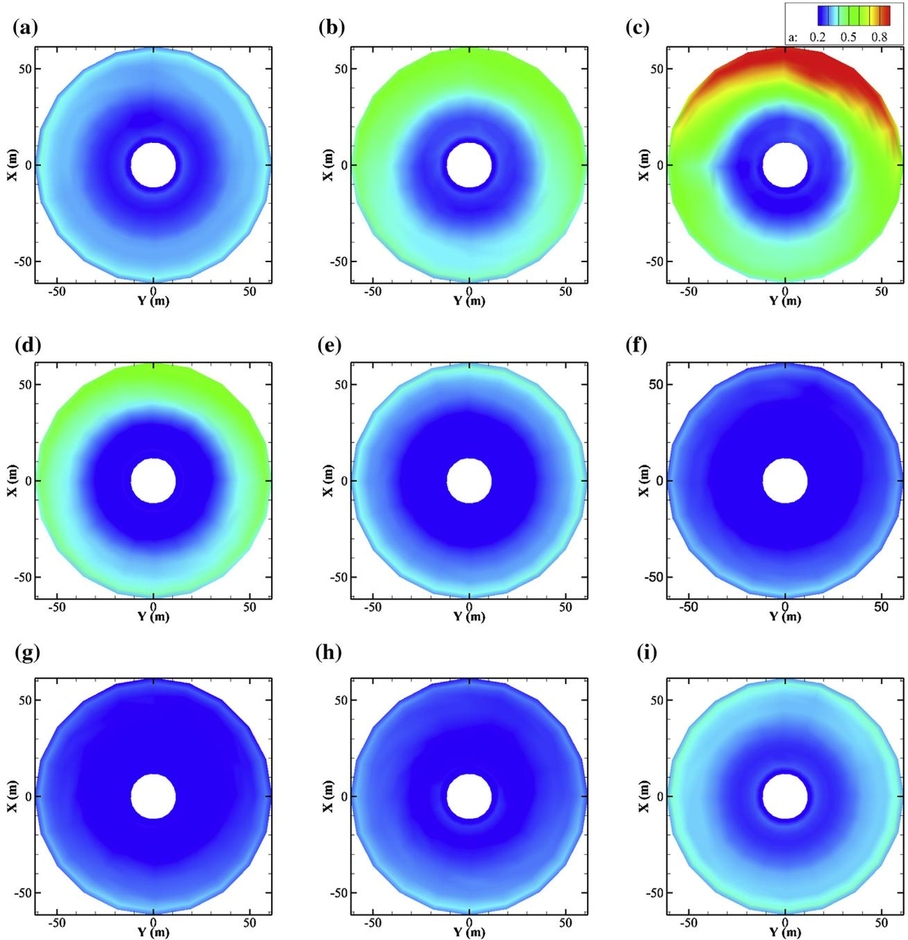
Fig. 6. Local induction factor at each platform pitching location – (a)–(i) : locations 1–9 in Fig. 4.
