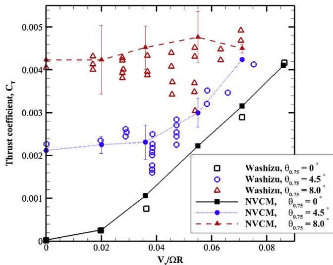
Fig. 2. Thrust coefficient versus vertical flight velocity factor for different values of the pitch angle when the blade section  $x$  equals 0.75.
