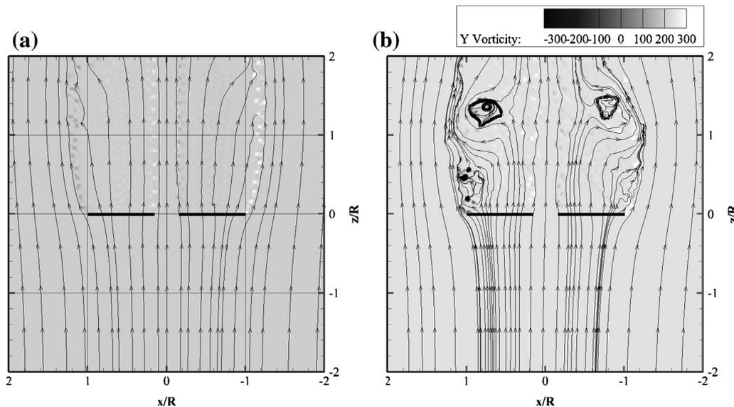
Fig. 5. Normal vorticity fields and streamlines at  $V_z = 4.5$  m/s – (a) fixed wind turbine, (b) floating wind turbine.
