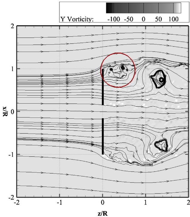
Fig. 8. Normal vorticity fields and streamlines of the floating wind turbine at location seven.
