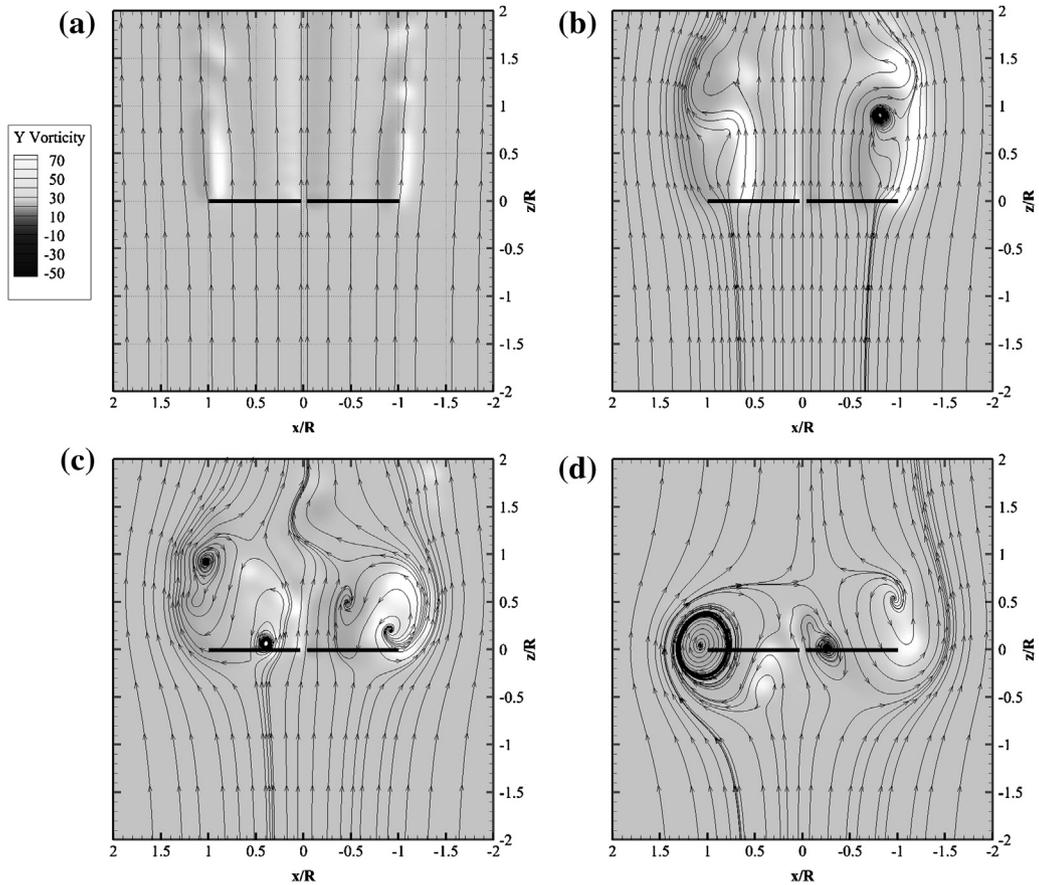
Fig. 3. Normal vorticity fields and streamlines at  $\theta_{0.75} = 4.5^\circ$  – (a)  $V_z = 6.6$  m/s, (b)  $V_z = 5.0$  m/s, (c)  $V_z = 3.2$  m/s, (d)  $V_z = 1.1$  m/s.
