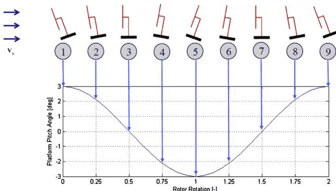
Fig. 4. Floating turbine stances during pitching motion.
